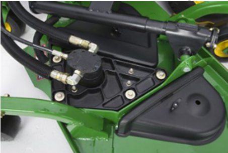
Isolated deck motor design
