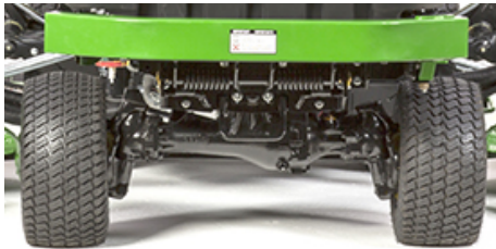
1600 Turbo Series III Wide-Area Mower (WAM) mechanical rear-wheel drive axle
