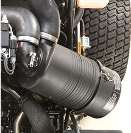
Air filter with air-restriction indicator
