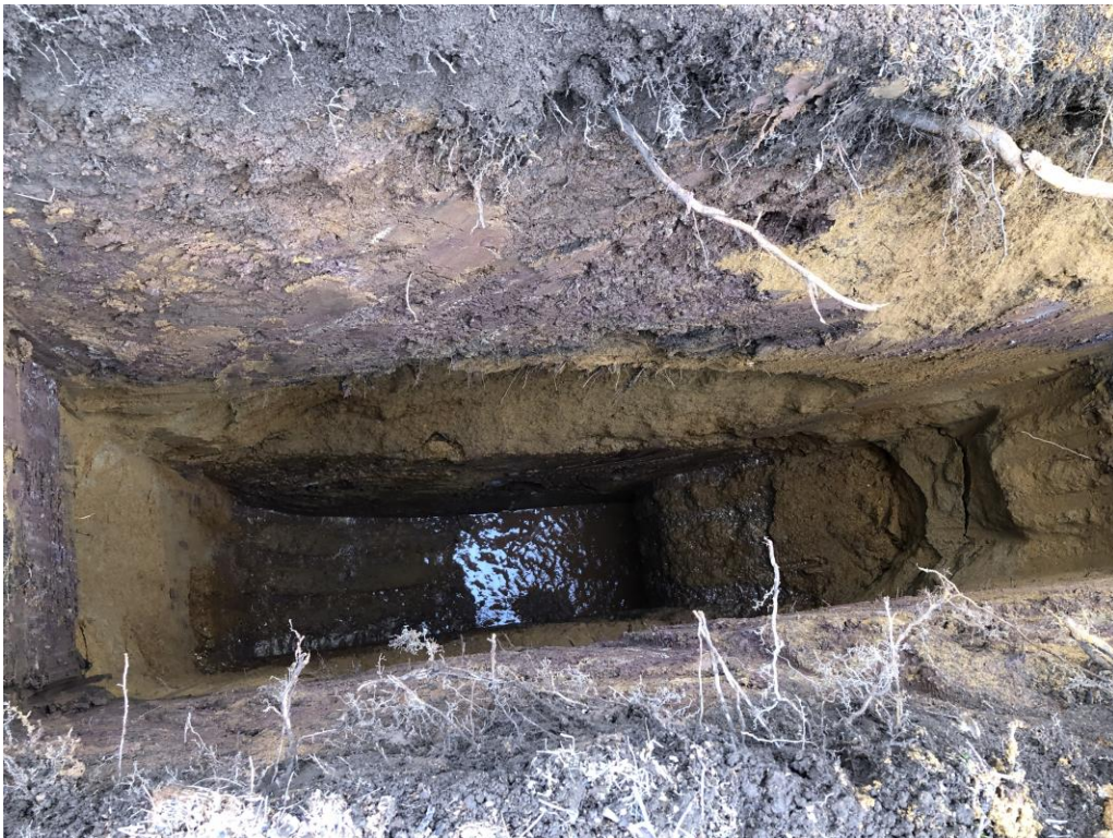
Photo 4: Profile of Test Pit STP-2.
