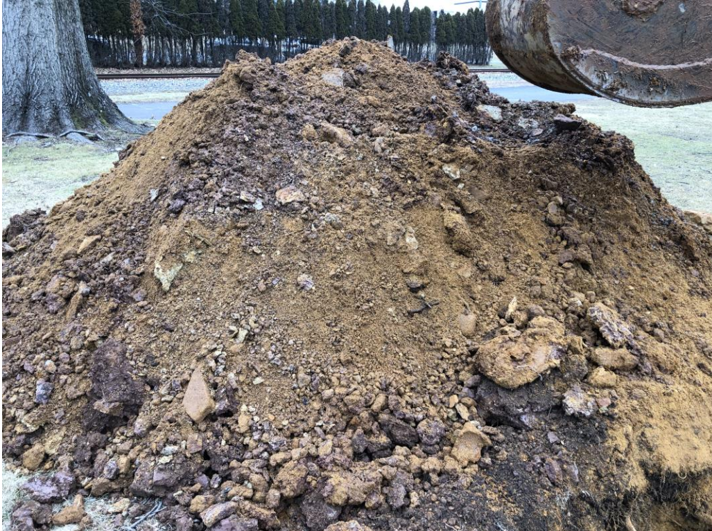
Photo 5: Excavated material from Test Pit STP-2.
