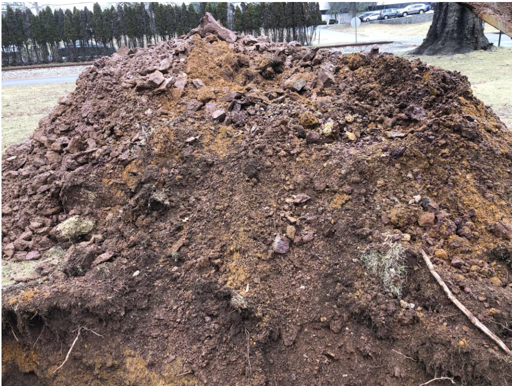
Photo 2: Excavated material from Test Pit STP-1.
