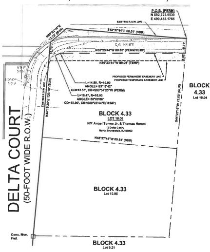
EXISTING AREA OF LOT 10.06 IN BLOCK 4.33 = 6,500 S.F. or 0.149 AC.± AREA OF PROPOSED PERMANENT EASEMENT = 1,177 S.F. or 0.027AC.± AREA OF PROPOSED TEMPORARY EASEMENT = 434 S.F. or 0.010 AC. ±
